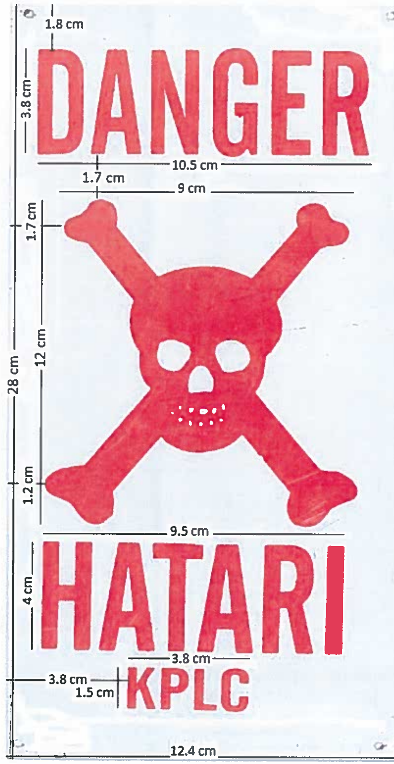
Fig. 3: Danger/Hatari plate for power lines
